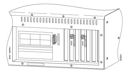
9 At the rear of the unit, connect the network cable for the external, Internet-connected network to the Ethernet adapter on the PIX Firewall labeled "Outside."
