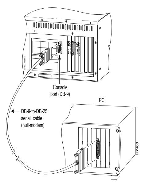
5 Configure the serial port in your computer or terminal with these settings: 9600 baud, 9 data bits, no parity, and 1 stop bit; that is, set 9600, 8-N-1. Ensure your communications software is running.
