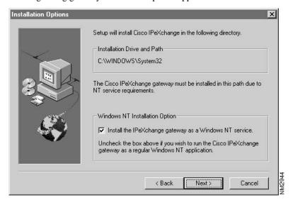
**Step 5** If you do not want the IPeXchange gateway to be installed as an NT service, deselect the checkbox.
