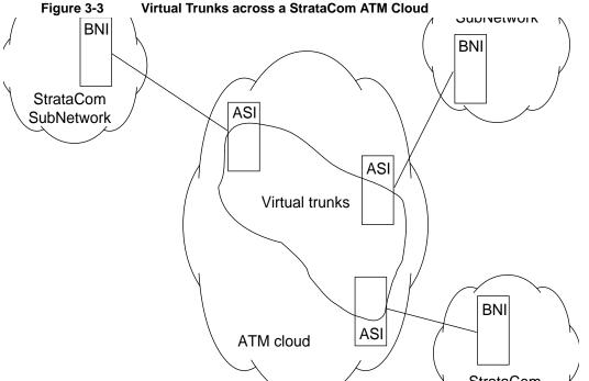
2 Configure the cloud ASI ports. For each ASI port connected to a BNI virtual trunk port, do the following:
