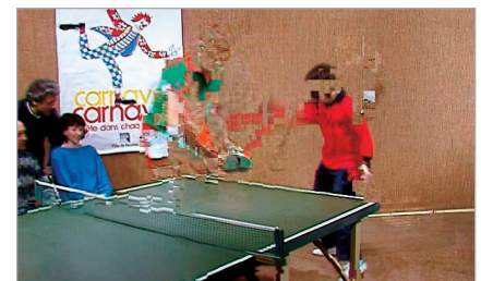
Figure 2. Ghosting. In this image, I-frame loss near a scene change continues to display the pre-scene-change image. As the decoder receives the P- and B-frames from the new group of pictures, it adds this new information to the old scene, creating the ghosting effect. (Source: the Society of Motion Picture Television Engineers; used with permission.)
